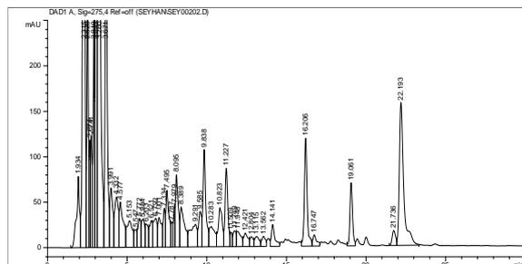
**Figure 3.** Chromatographic separation of *K. vermilio* hydrolyzed extract by HPLC with UV-visible detection at 275 nm. *K. vermilio* pigments: minor dyestuffs are designated yellow and red, flavokermesic acid, Rt:21.73, and kermesic acid, Rt:22.19.
