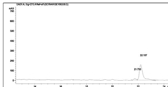
**Figure 1.** Chromatogram of the standard dyestuff mixture at 275 nm. flavokermesic acid, Rt:21.73; kermesic acid, Rt:22.18.
