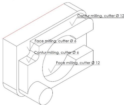
**Figure 11. Part surfaces used for determining the roughness value**
