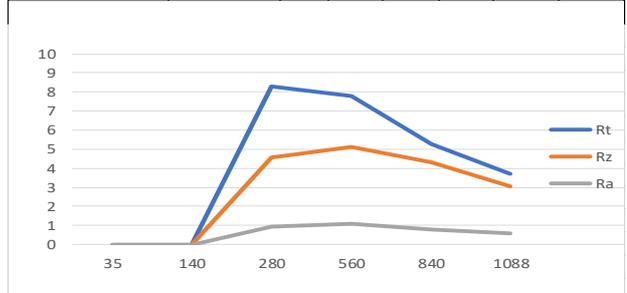
Figure 14. Roughness values for PLA parts after the machining with the  $\varnothing 6\text{mm}$  end mill
