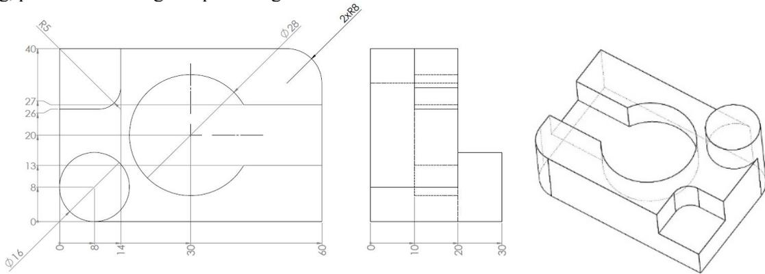
**Figure 4 Specimen design and milling dimensions**
