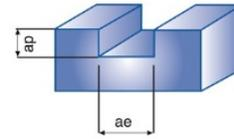
$V_c$  – Cutting speed(m/min); D –Cutter diameter (mm); n – Spindle speed (rev/min);  $V_f$  – Feed speed;  $f_z$  – Feed per tooth(mm/tooth); f – Feed per rev(mm/rev); z – Number of teeth; ap -depth of cut; ae – width of cut; K – Correction coefficient.
