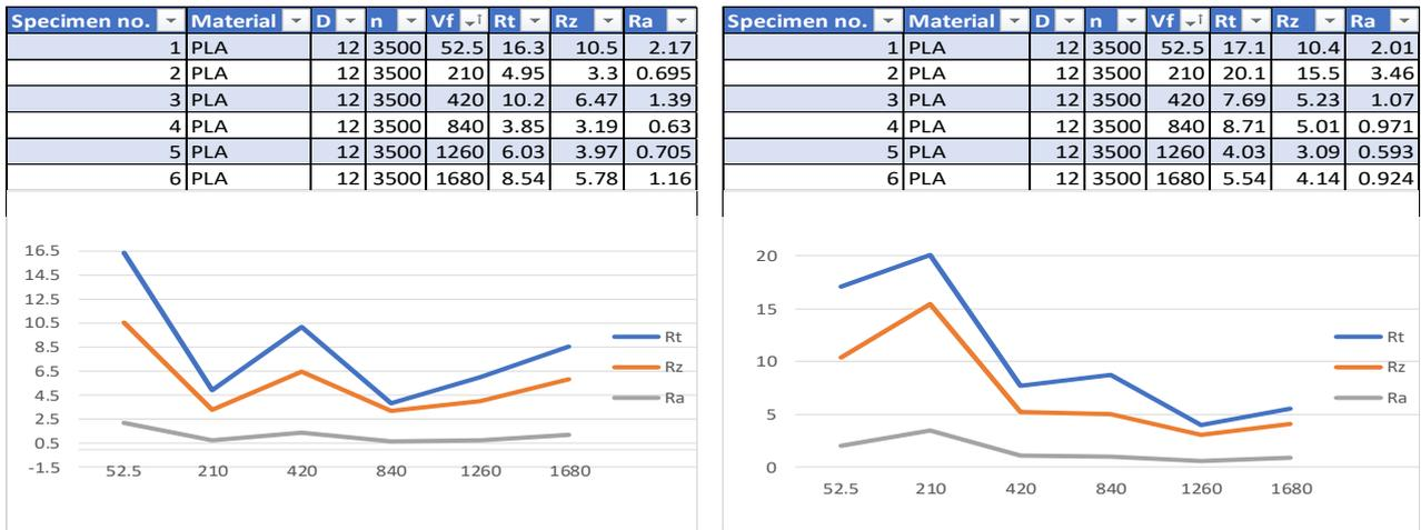
Figure 15. Roughness values for PLA parts after the machining with the  $\varnothing 12\text{mm}$  end mill
