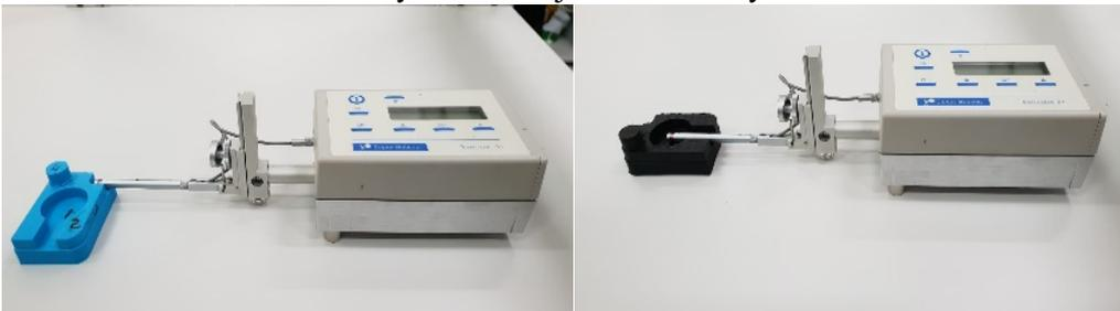
**Figure 9. Roughness measurement with “Taylor Hobson Surtronic 3+” measuring probe**
