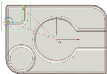
**Figure 6.  $\phi 6$  mm end mill climb trajectory**
