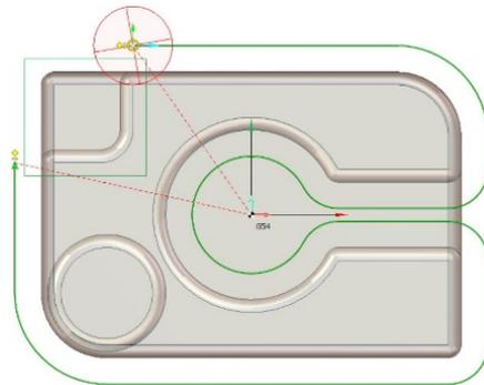
**Figure 7.  $\phi 12$  mm end mill climb trajectory**
