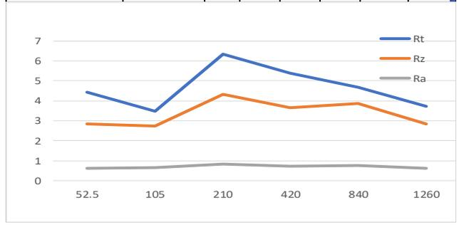
Figure 13. Roughness values for ABS parts after the machining with the  $\varnothing 12\text{mm}$  end mill
