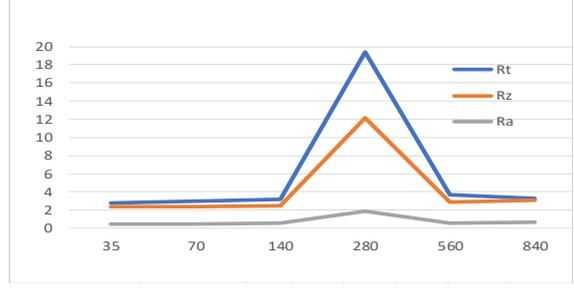
Figure 12. Roughness values for ABS parts after the machining with the  $\varnothing 6\text{mm}$  end mill
