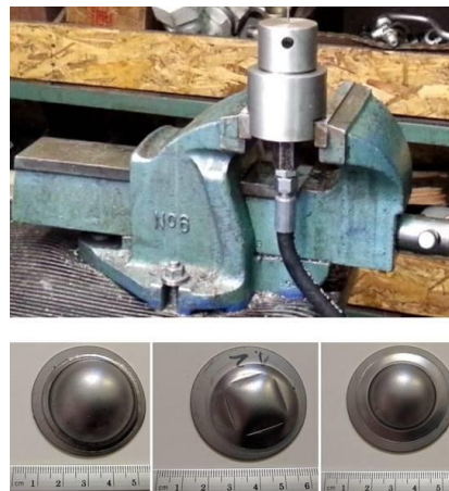
Figure 8: Developed die and hydroformed parts
