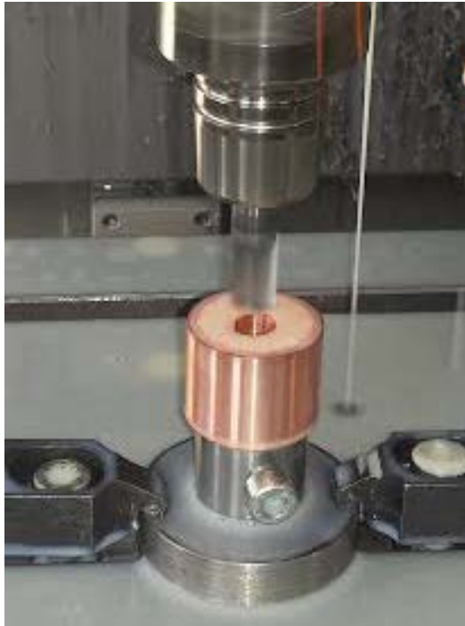
Figure 11: Roughing operation with 12 mm end mill
