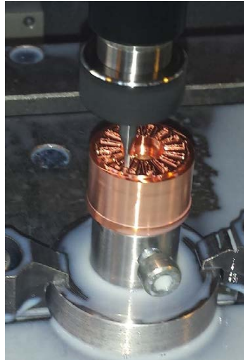
Figure 12: Roughing operation with 2 mm end mill
