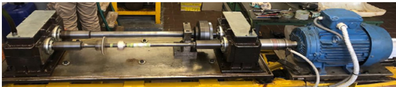
Fig. 1 Niemann M01 FZG back-to-back test rig
