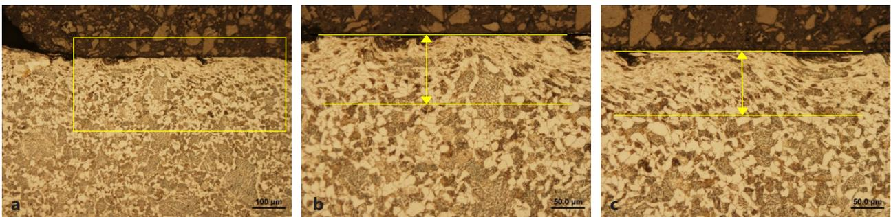
**Fig. 9** Plastic deformation (0.13–0.18 mm) on the face place of the tool
