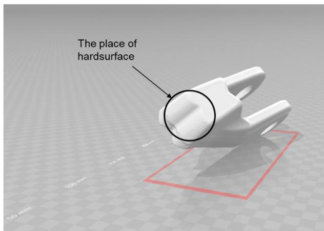
**Fig. 13** Recommended place for application of hardfacing
