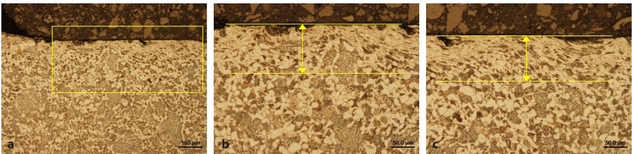
**Fig. 8** Plastic deformation at up to 0.12 mm on the face place of the tool
