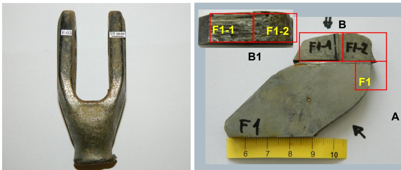
**Fig. 6** Preparation of samples for metallographic analysis
