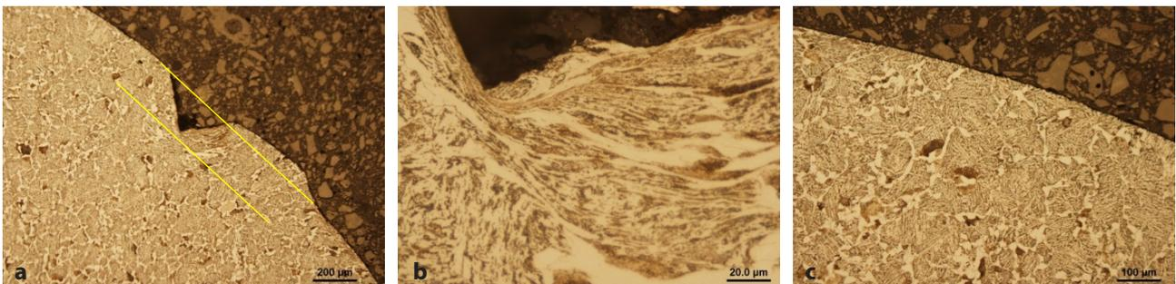
**Fig. 10** 0.2 mm plastic deformation on the face place of the tool
