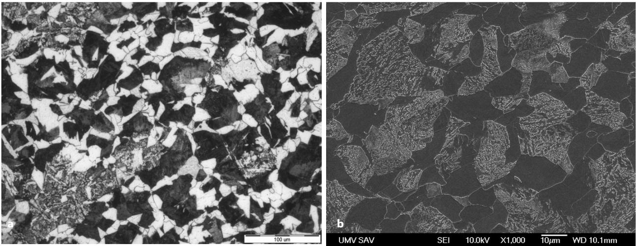
**Fig. 7** Detail of the tool body microstructure – a) light microscope; b) scanning electron microscope (SEM)
