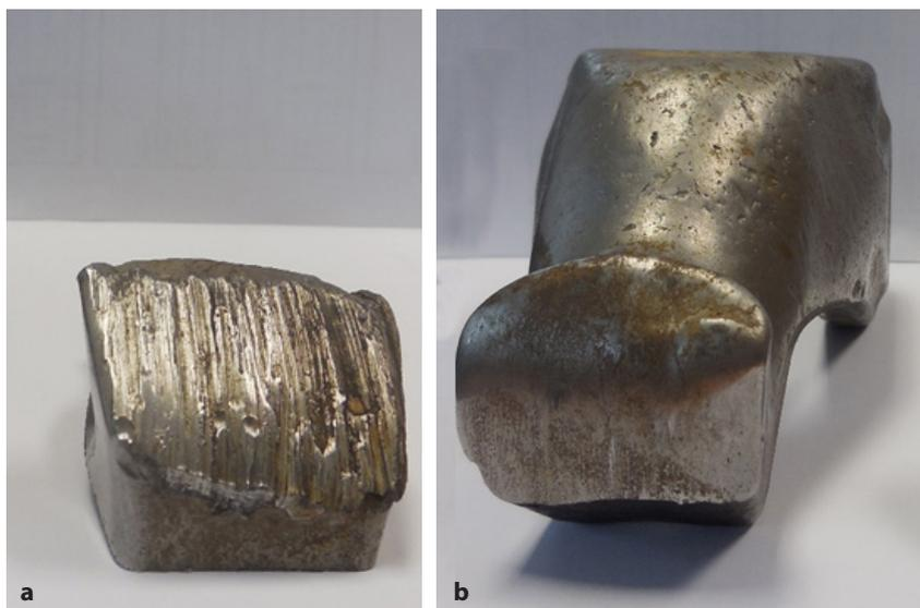
**Fig. 3** Tool wear after loss of WC tips
