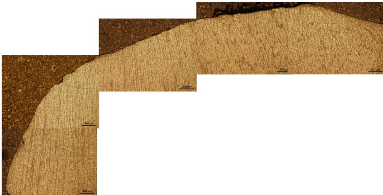
**Fig. 11** Profile of the worn tool face
