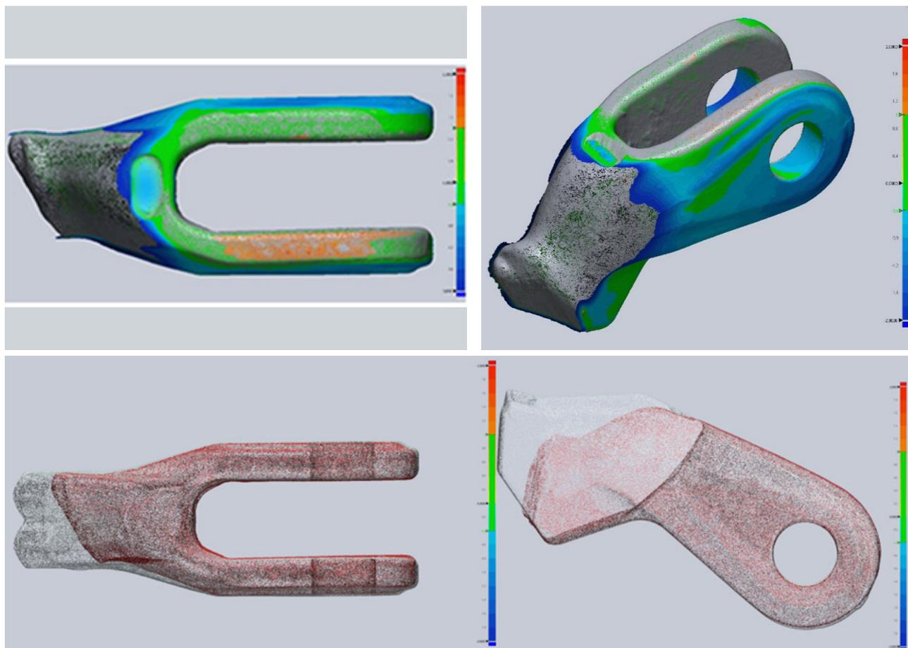
**Fig. 5** Deformation and loss of tool material in a 3D scan
