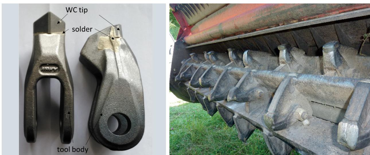
**Fig. 2** Tools and roller with working tools
