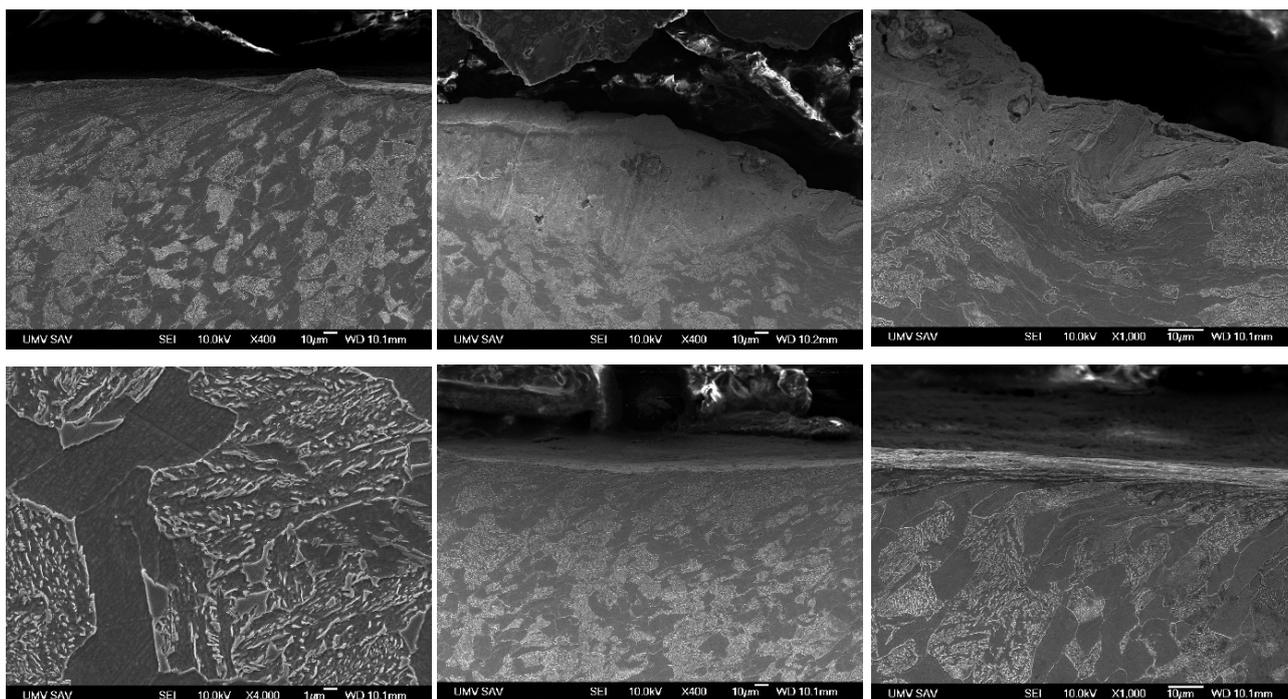
**Fig. 12** SEM surface of the worn tool
