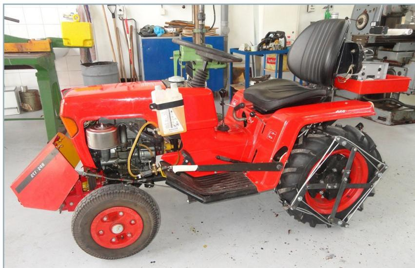
**Fig. 1** The tractor type Mini 070 equipped with prototypes of driving wheels
