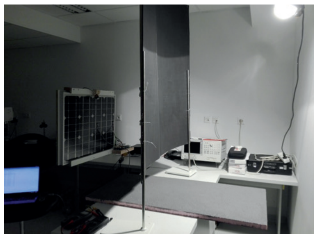
Fig. 4 Measurement of PV module power with shutter – measurement no. 2
