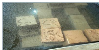
Figure 4b Curing tank 2
