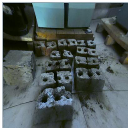
**Figure 11** Cracked bricks during M.O.R. test
