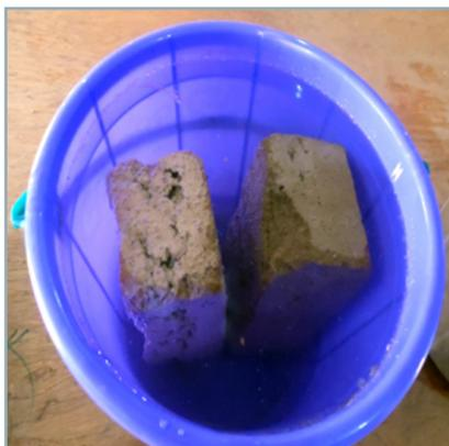
**Figure 6** Immersion in water
