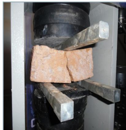
**Figure 10** M.O.R. test
