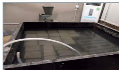
Figure 4a Curing tank 1
