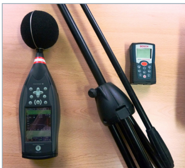
Figure 2 From the left to the right: Measuring device Brüel & Kjær type 2270 with a tripod and digital distance meter Bosch DLE 50
