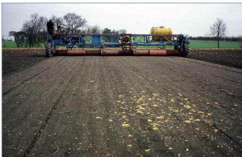
**Figure 2** Mounted rolls were designed for this 12 m wide span vehicle at Silsoe. Precise firming was applied by transferring weight from the vehicle to the rolls using hydraulic pressure
