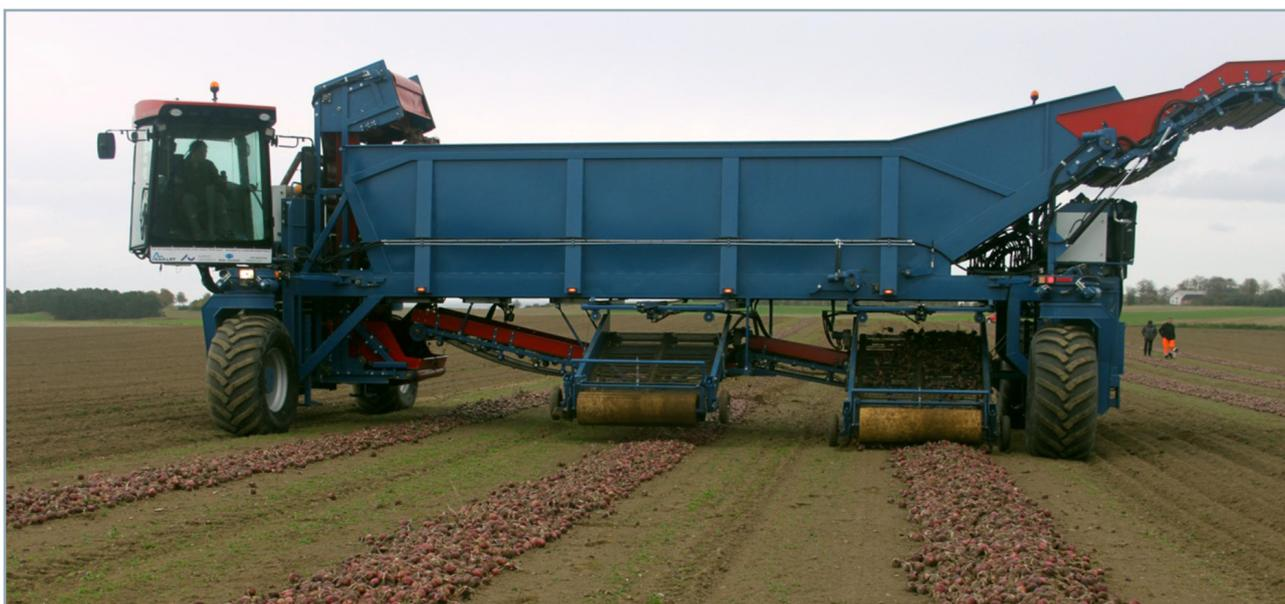
**Figure 4** The ASA-Lift WS9600 wide span vehicle loading onions on a farm in Denmark. This machine presently integrates with a tractor-based system using tractors with a 3.2 m track gauge
