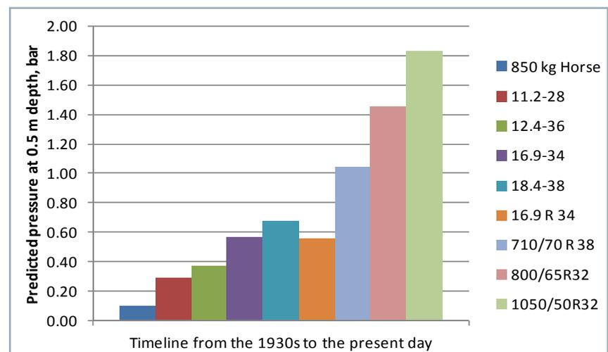
**Figure 1** Change in soil stress at 0.5 m depth predicted for different loads and pressures at the surface under a horse and under tyres of increasing size
