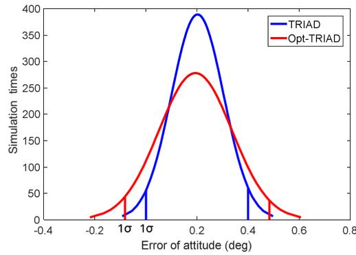
Fig. 1. Simulation results of attitude determination in the same accuracy case
