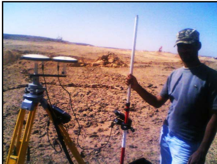
Fig. 2. Initialization by bar setup at Reference point
