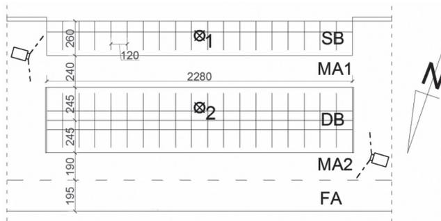
Figure 1. Projection of the tested area with marked locations of measurement and observation cameras; 1, 2 – measurement points of temperature, relative humidity and air velocity, SB – single boxes, DB – double boxes, MA1, 2 – manure alleys, FA – feeding and manure alley
