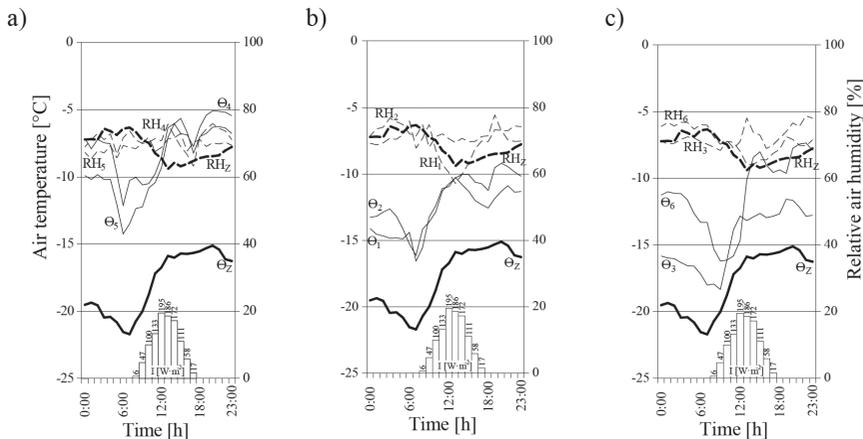
Figure 4. Temperature ( $\Theta_z$ ,  $\Theta_{1-6}$ ), relative air humidity ( $RH_2$ ,  $RH_{1-6}$ ) and solar radiation intensity ( $I$ ) on a cloudy day of 4 February 2012 inside the barn in Kobylny for three technological groups; a) group 1, b) group 2, c) group 3 (own source)
