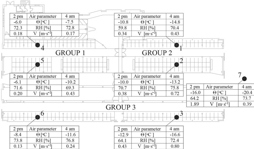
Figure 7. Layout of the building with measurement points (1–7) and hourly average values registered on 4 February 2012 at 4 am and 2 pm (own source)
