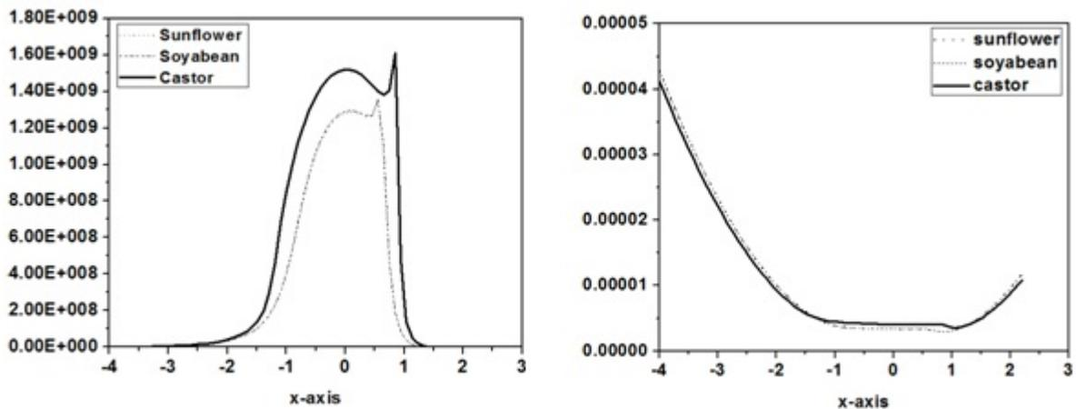
**Fig. 3** EHL pressure and film thickness profile for all tested oils.  $U = 1.0 \times 10^{-11}$  and  $W = 2.0452 \times 10^{-5}$ .
