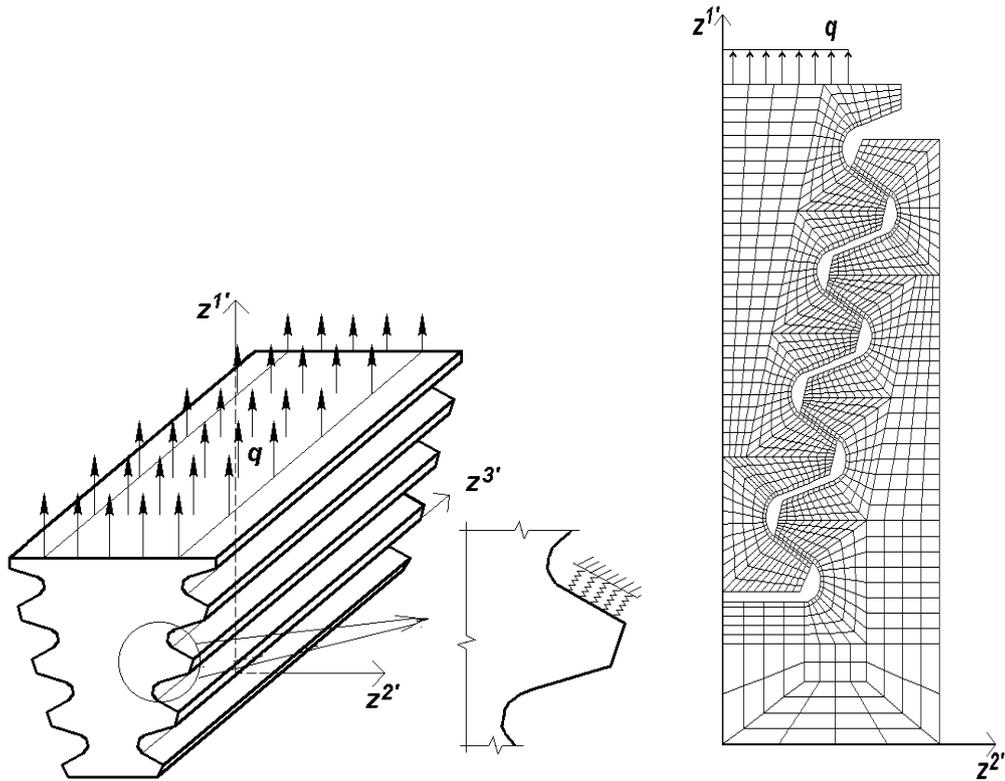
Fig. 4 Root of gas turbine blade: design scheme (left) and SFEM discrete model.
