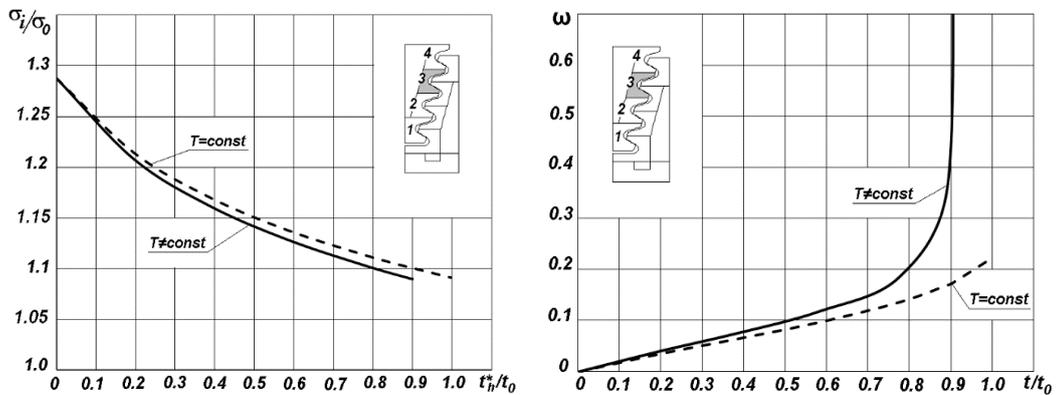
Fig. 5 Change in time of dimensionless stress intensity (left), and damage parameter.
