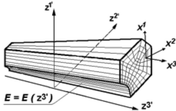
Fig. 2 SFEM discrete model of prismatic inhomogeneous body.
