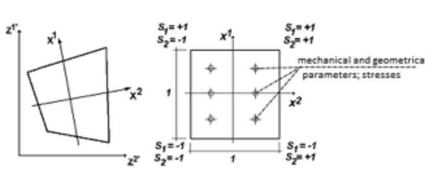
Fig. 1 Two-dimensional finite element in general (left) and local coordinate system.
