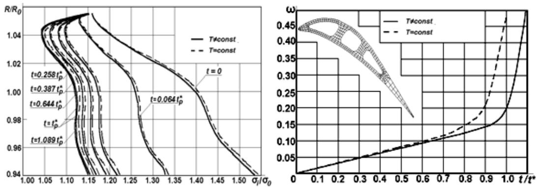
Fig. 7 Changing of stresses across the height of the blade (left), time-dependent damage parameter values.
