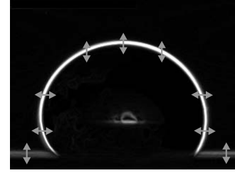
Fig. 13. Direction of gradient profile reconstruction in different parts of the specimen profile.
