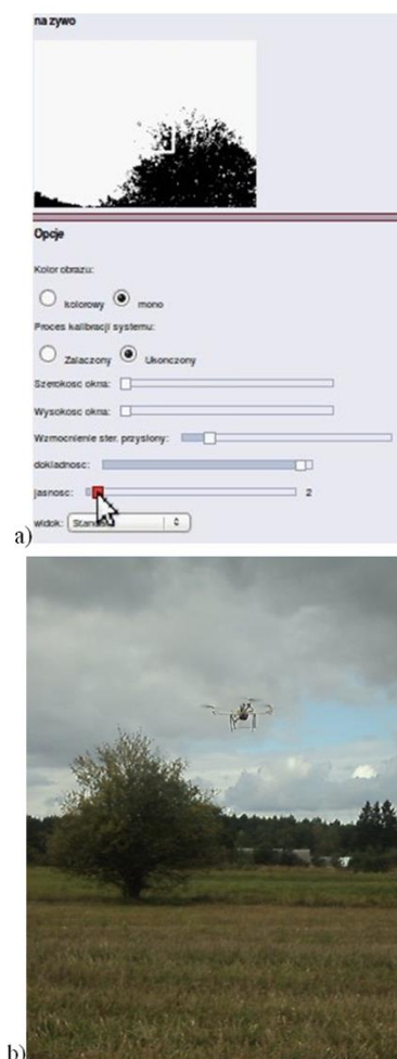
Fig. 9. Field experiments: a) picture from the webserver of vision system b) photo of the tree as an obstacle (made during the field test)
