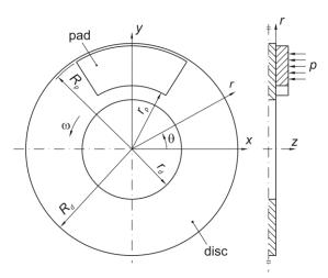
Fig. 1. A schematic diagram of a pad-disc brake system
