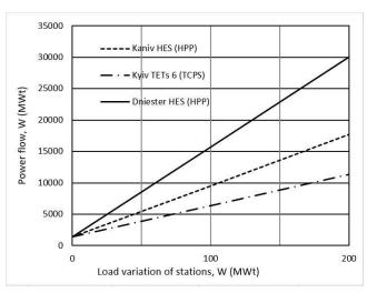
Fig. 3. Experiment data of the impact of generating stations on power flow at South-Ukraine Nuclear Power Plant-Vinnitsa
