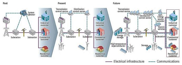
Fig. 1. Transition of power system architecture into smart one
