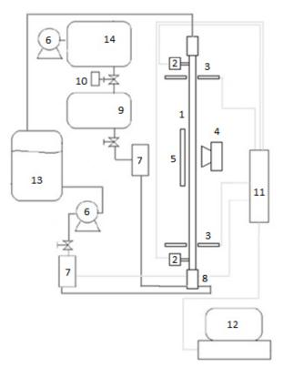
Fig. 1. Experimental setup: 1 – vertical minichannel with a diameter of 3 mm, 2 – pressure sensors (MPX12DP), 3 – laser-phototransistor sensor, 4 – Phantom v. 1610 camera, 5 – lighting, 6 – pumps (air or water), 7 – flow meters, 8 – mini bubbles generator, 9 – air tank, 10 – automatic valve to maintain a constant pressure in the tank 9, 11 – data acquisition station (DT9800), 12 – computer, 13 – water tank, 14 – air tank
