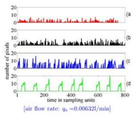
Fig. 5. Time series in terms of number of pixels xi passing through the gate in the central cross-section of the camera view (Fig. 1). The cases presented downward correspond to (a)–(d) in Fig. 2. The sampling time step was  $0.2 \times 10^{-3}$  s. Number of points (range of horizontal axis) was 800.
