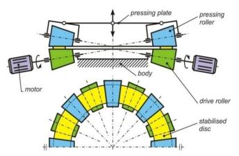
Fig. 3. Schematic diagram of the station for the dynamic stabilisation of friction discs
