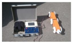
Fig. 16. The pipe inspection robot prototype and the control panel
