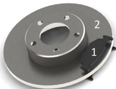
**Fig. 1.** Brake pad (1) and corresponding brake disc (2) – CAD model developed for the purpose of this paper based on manufacturer data
