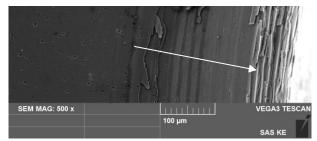
**Fig. 12.** Punch – surface in the edge of R0.5 and decohesion of ZrN coating
