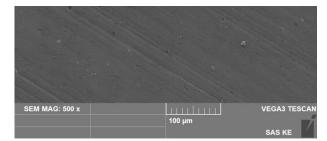
Fig. 5. ZrN coating after deposition SEM
