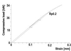
Fig. 14. Compression test of punch-Ø5x4 mm
