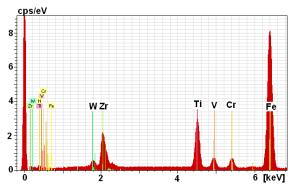
Fig. 8. EDX microanalysis in the edge of R0.5
