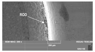
Fig. 9. Die – defect in the radius surrounding the cavity of shaped surface ROD
