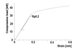
Fig. 13. Compression test of punch- Ø3.6x2.1 mm
