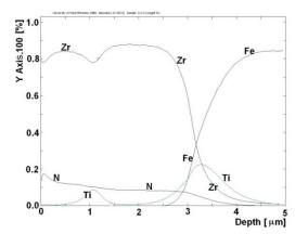
Fig. 3. GD-OES. ZrN coating, substrate 1.3343, 55 HRc
