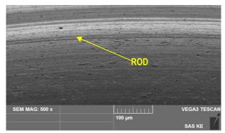
Fig. 10. Die – radius of surrounding of cavity of shaped surface – ROD, after deposition of ZrN coating
