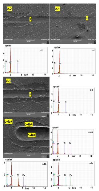
Fig. 19. ZrN – detail of the coating failure and qualitative EDX microanalysis in positions 1,2,3,4 from Fig.18.
