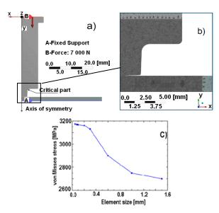
Fig. 15. Defined a) boundary conditions, b) finite element mesh, c) optimization of mesh
