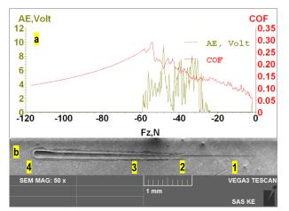
Fig. 18. ZrN, a) record AE-Fz, COF-Fz, b) scratch – disposition
