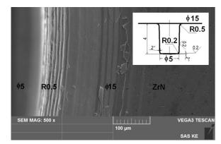
**Fig. 7.** Decohesion of ZrN coating in the edge of R0.5
