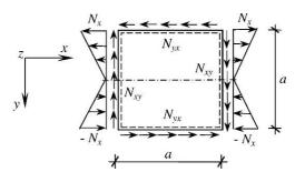
Fig. 5. Considered element of the steel welded girder
