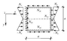
Fig. 7. Considered element of the steel welded girder
