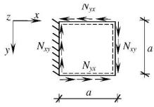
Fig. 3. The plate subjected to in-plane tangential loading
