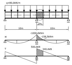
Fig. 16. Analysed steel welded-girder
