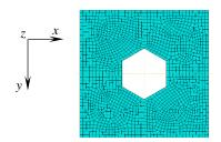
Fig. 14. Considered element of steel welded girder with hexagonal hole
