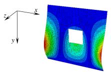
**Fig. 11.** The first buckling mode for simply-supported square plate with square hole  $(\tilde{N}_{xy}/\tilde{N}_x=0)$
