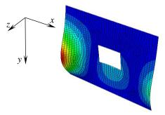
**Fig. 12.** The first buckling mode for simply-supported square plate with square hole  $(\tilde{N}_x/\tilde{N}_x=0.025)$
