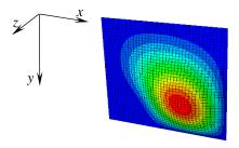
Fig. 6. The first buckling mode for simply-supported square plate  $(\tilde{N}_{xy}/\tilde{N}_x=0.1)$
