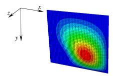
Fig. 8. The first buckling mode for square plate clamped along one edge and simply-supported along other edges  $(\tilde{N}_{xv}/\tilde{N}_x = 0.1)$
