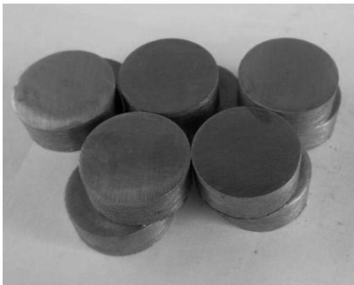
**Fig. 2.** Examples of samples prepared for ball-cratering tests
