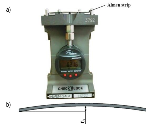
**Fig. 1.** Photo of Almen gage TSP-3 (a) and scheme of Almen strip after shot peening (b)
