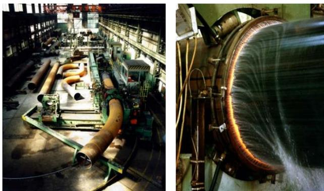
Fig. 1. Description of induction bending machine (left) and the induced zone where bending takes place (right) (Muthmann and Grimpe, 2006)
