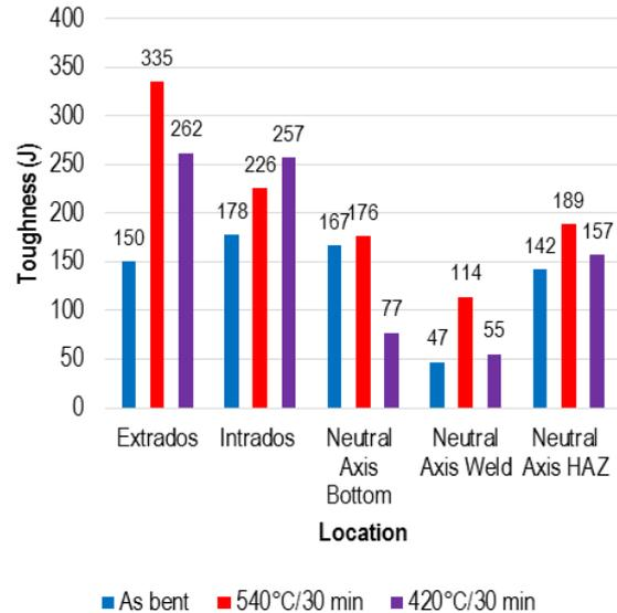
Fig. 12. Toughness values of the bend zone
