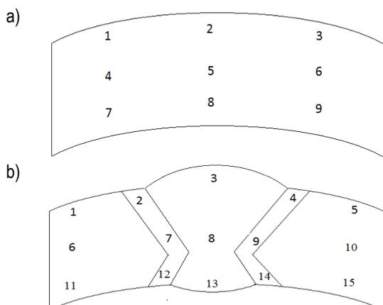
Fig. 7. Drawings of samples for hardness measurement; a. seamless, b. with weld
