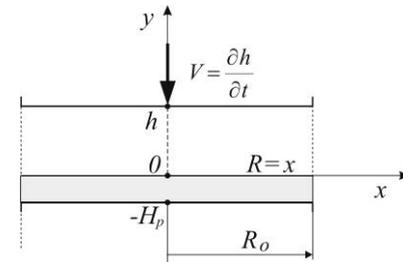
Fig. 3. Squeeze film in a radial thrust bearing
