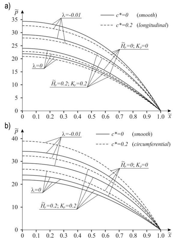
Fig. 4. Dimensionless pressure distribution in the squeeze film thrust bearing with rough surfaces for  $\tilde{H}_p = 0.2$ ,  $K_p = 0.2$ ,  $\lambda = -0.01$  and  $\lambda = 0$  and  $\varepsilon = 0.5$ ; (a) longitudinal roughness and (b) circumferential roughness
