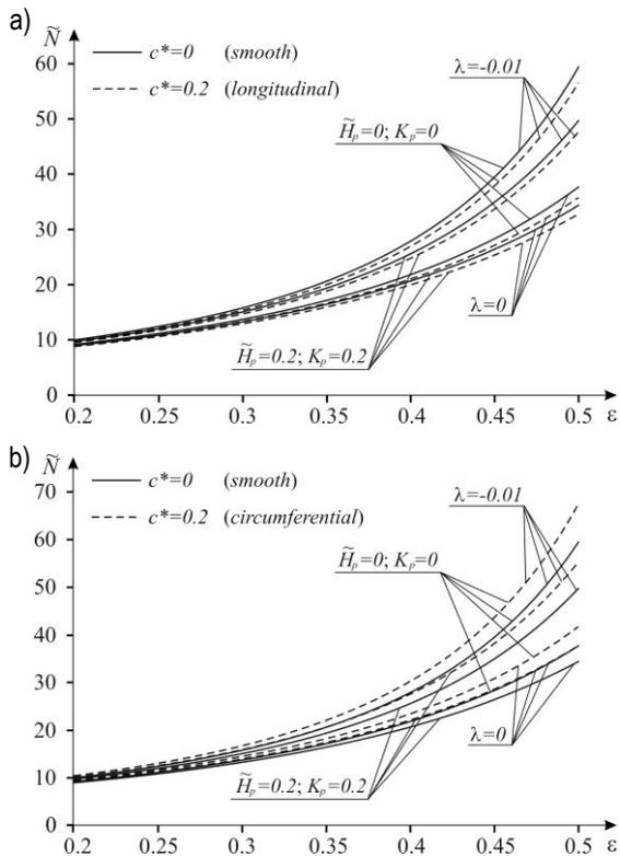
Fig. 6. Load-carrying capacity for the squeeze film thrust bearing with rough surfaces for  $\tilde{H}_p = 0.2, K_p = 0.2, \lambda = -0.01$  and  $\lambda = 0$  and  $\epsilon = 0.5$ ; (a) longitudinal roughness and (b) circumferential roughness
