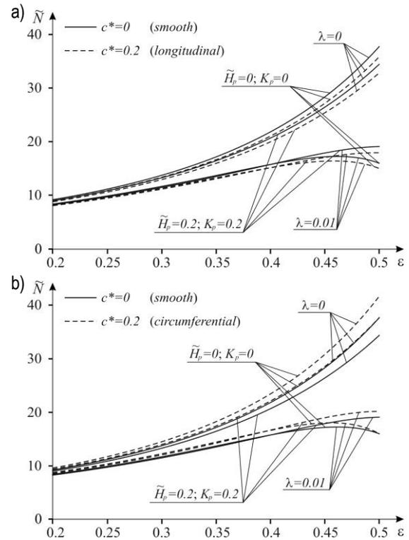
Fig. 7. Load-carrying capacity for the squeeze film thrust bearing with rough surfaces for  $\tilde{H}_p = 0.2, K_p = 0.2, \lambda = 0$  and  $\lambda = 0.01$  and  $\epsilon = 0.5$ ; (a) longitudinal roughness and (b) circumferential roughness
