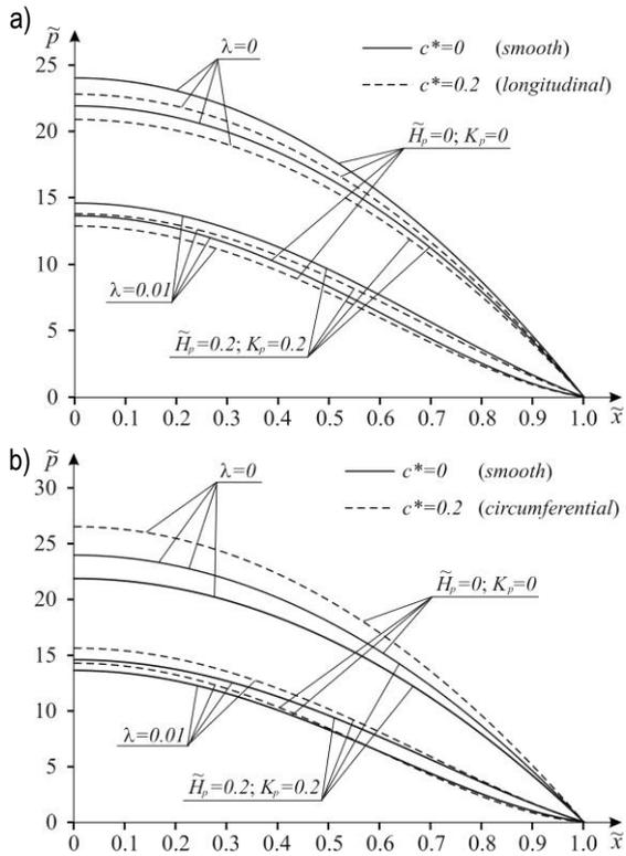
Fig. 5. Dimensionless pressure distribution in the squeeze film thrust bearing with rough surfaces for  $\tilde{H}_p = 0.2, K_p = 0.2, \lambda = 0$  and  $\lambda = 0.01$  and  $\epsilon = 0.5$ ; (a) longitudinal roughness and (b) circumferential roughness
