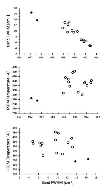
**Figure 5:** Representative example showing the apatite band parameters of the conodont sample 5. Reliable RSCM temperature estimates (full circles) are recorded by spot measurements with a v<sub>1</sub>-PO<sub>4</sub> parameter combination of band center < 956 cm<sup>-1</sup> and band FWHM > 12cm<sup>-1</sup> (corrected temperatures of Table 3).
