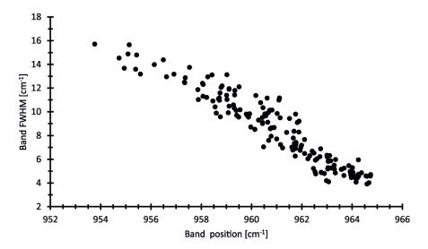
**Figure 4:** Relationship between band width (FWHM= full width at half maximum) and position of the v1-PO<sub>4</sub> band as estimated on 180 condont spot locations (all recorded spot data are shown). The covariation indicates a continuous variation of the substituting ion concentration in the apatite lattice (Thomas et al., 2011).
