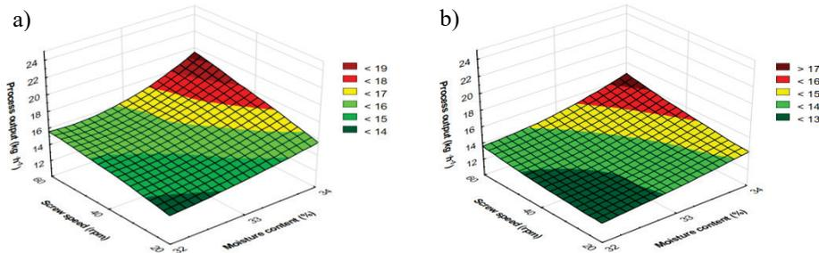
Figure 1. Effect of processing variable conditions on processing efficiency during the extrusion of various raw materials: a) potato composition, b) multigrain composition
