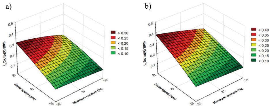
Figure 2. Effect of processing variable conditions on specific mechanical energy requirements during the extrusion of various formulations of raw materials: a) potato composition, b) multigrain composition
