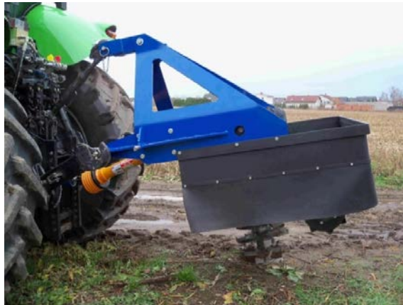
Figure 2. Model of a new machine for cutting willow rootstocks as well as bushes and young trees
