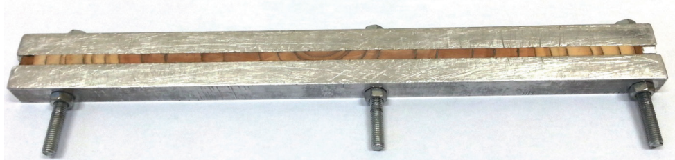
Figure 4. A sample placed in a special aluminium grip. (photo R. Wąsik)
