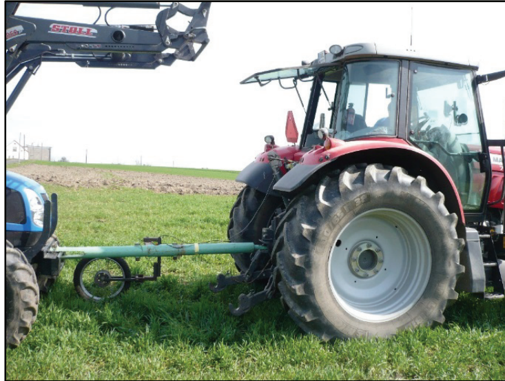
Fig. 2. Measurement stand consisting of two tractors connected with a tow rod
