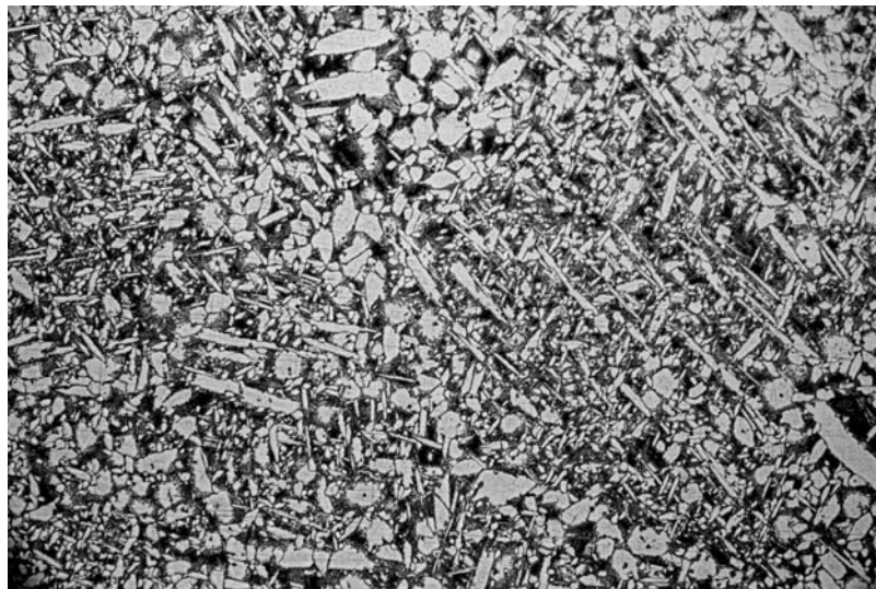
Fig. 1. Microstructure of BA1055 bronze. White grains - \alpha phase, dark fields - eutectoid \alpha+\gamma_2 , \kappa -phase – slightly visible. Magn. 200x
