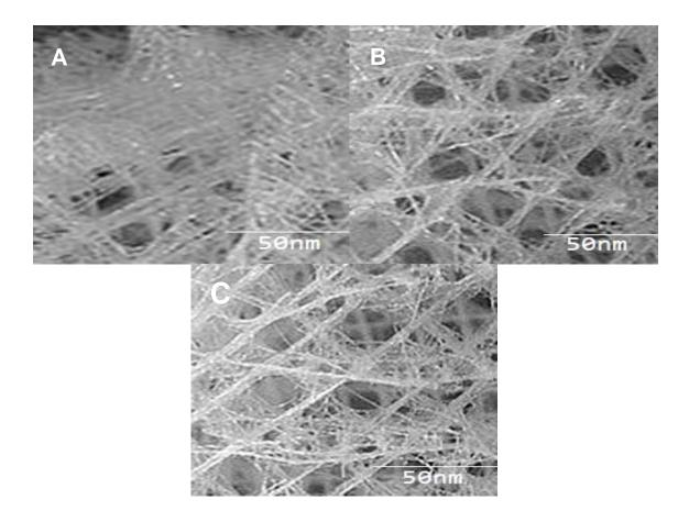
Fig. 4. TEM micrographs of (A) PAN/PS Foam; (B) PAN/PS/CNP 0.3 Foam; and (C) PAN/PS/CNP 3 Foam
