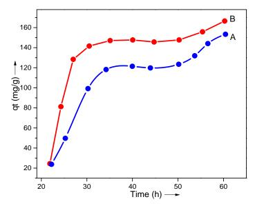
Fig. 9. Time-dependent amount (qt) of Pb2+ ions removed by (A) PAN/PS/CNP 0.3 Foam and (B) PAN/PS/CNP 3 Foam in aqueous solutions with initial Pb2+ ion concentration of 100 mg/L at pH 3
