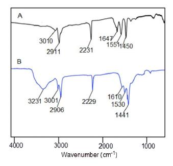
Fig. 2. FTIR spectra of (A) PAN/PS and (B) PAN/PS/CNP 3 Foam
