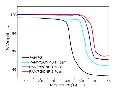
Fig. 7. TGA curves of PAN/PS and PAN/PS/CNP nanocomposite foam at 10 °C/min (N2)
