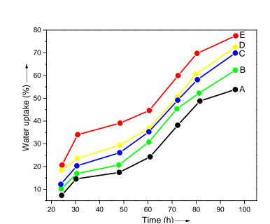
Fig. 8. Water uptake characteristics of (A) PAN/PS Foam; (B) PAN/PS/CNP 0.1 Foam; (C) PAN/PS/CNP 0.3 Foam; (D) PAN/PS/CNP 1 Foam; and (E) PAN/PS/CNP 3 Foam
