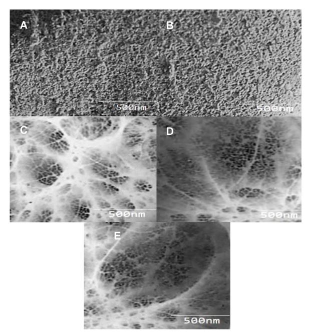
Fig. 3. FESEM micrographs of (A) PAN/PS Foam; (B) PAN/PS/CNP 0.1 Foam; (C) PAN/PS/CNP 0.3 Foam; (D) PAN/PS/CNP 1 Foam; and (E) PAN/PS/CNP 3 Foam
