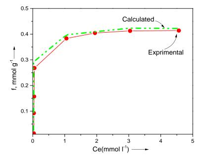
Fig. 10. Adsorption isotherms of Pb2+ ions for PAN/PS/CNP 3 Foam
