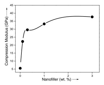
Fig. 6. Compression modulus of PAN/PS Foam and PAN/PS/CNP Foam
