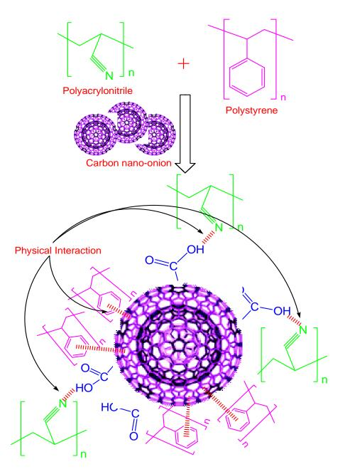
Fig. 1. Schematic for the formation of PAN/PS and CNP nanocomposite
