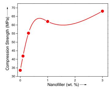
Fig. 5. Compression strength of PAN/PS Foam and PAN/PS/CNP Foam
