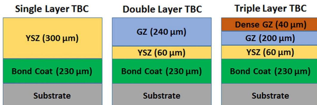
**Fig. 17.** Scheme of single- or multi-layered TBC manufactured by SPS [89]
