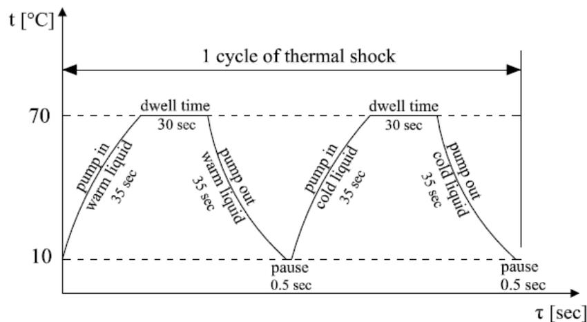
**Fig. 3.** Operating cycle of the thermal shock simulator
