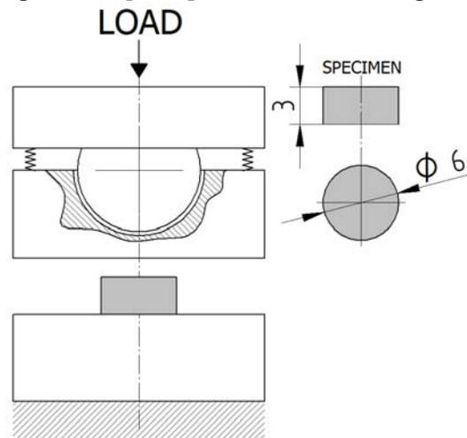
**Fig. 1.** Compressive strength test
