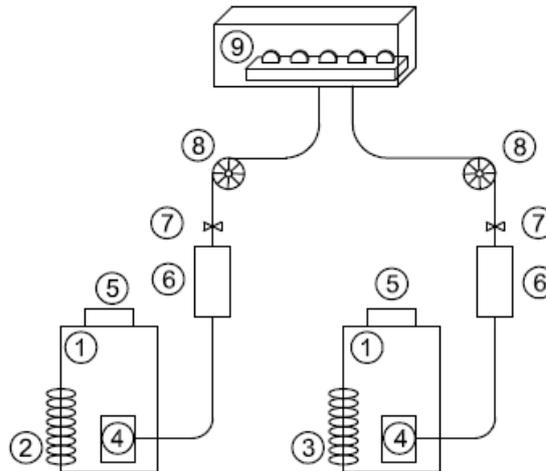
**Fig. 2.** Schematic of the hydraulic system of the thermal shocks simulator: 1 – working liquid tank, 2 – heating system, 3 – cooling system, 4 – rotary pump, 5 – thermostat, 6 – container, 7 – shut-off valve, 8 – peristaltic pump, 9 – specimen-holding vessel
