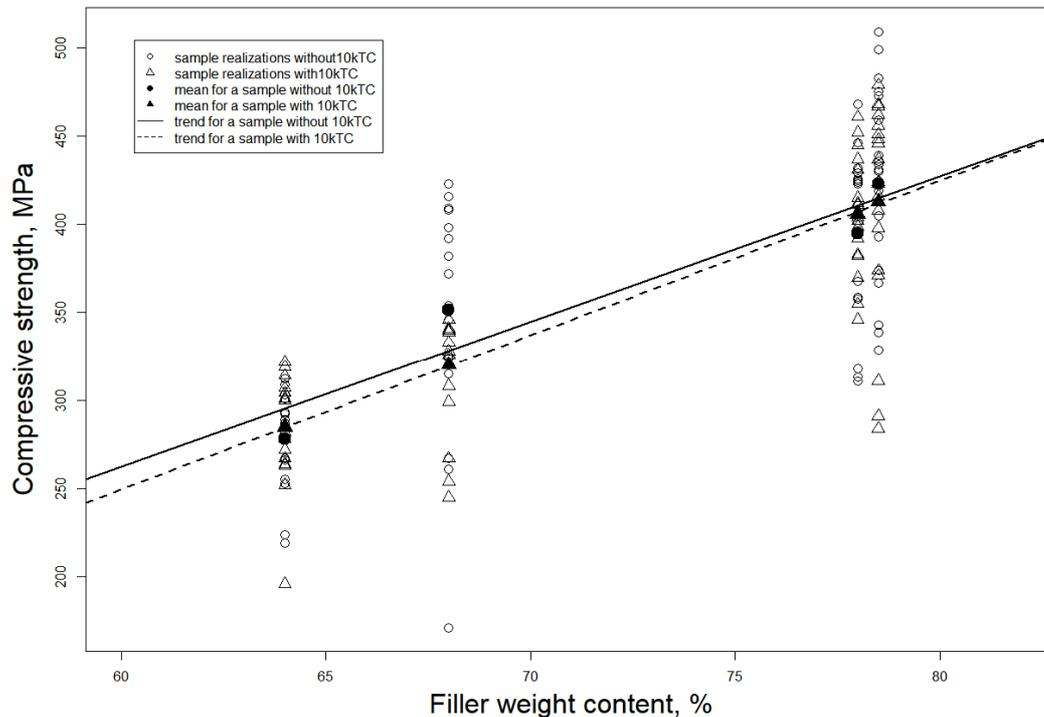
Fig. 4. Influence of filler content on the compressive strength of LC PMCCs
