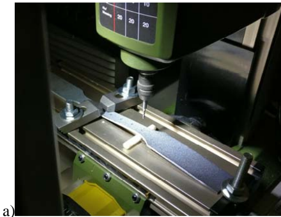
Fig. 3. Sample in a) convex and b) concave loading mode after hole drilling
