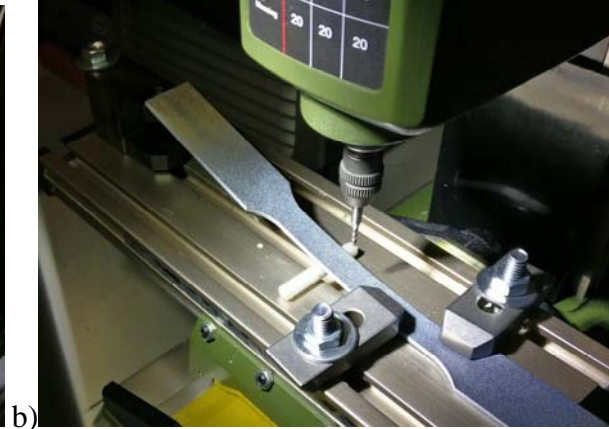
Fig. 3. Sample in a) convex and b) concave loading mode after hole drilling
