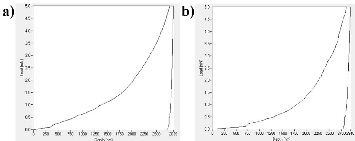
**Fig. 5.** Nanoindentation load-displacement curves carried out on the (a) nanoHAp and (b) nanoHAp/nanoAg coatings after thermal treatment
