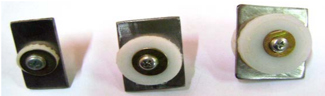
Fig. 1. Components of the multiple crevice assembly for corrosion test
