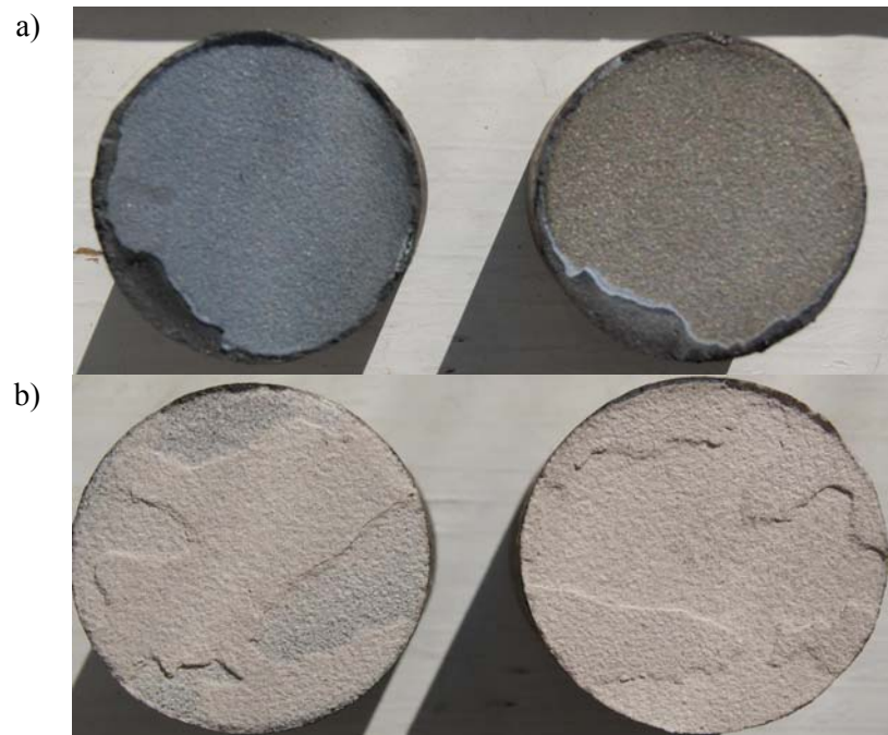
Fig. 15. The examples of fractures of samples with coatings sprayed with 97%Al 2 O 3 +3%TiO 2 powders and 70%ZrO 2 +30%CaO powders after static tensile test: a) sample 1/1, b) 2/1, (Table 5)
