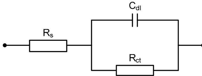
**Fig. 2.** The selected replacement of corrosion electrical circuit
