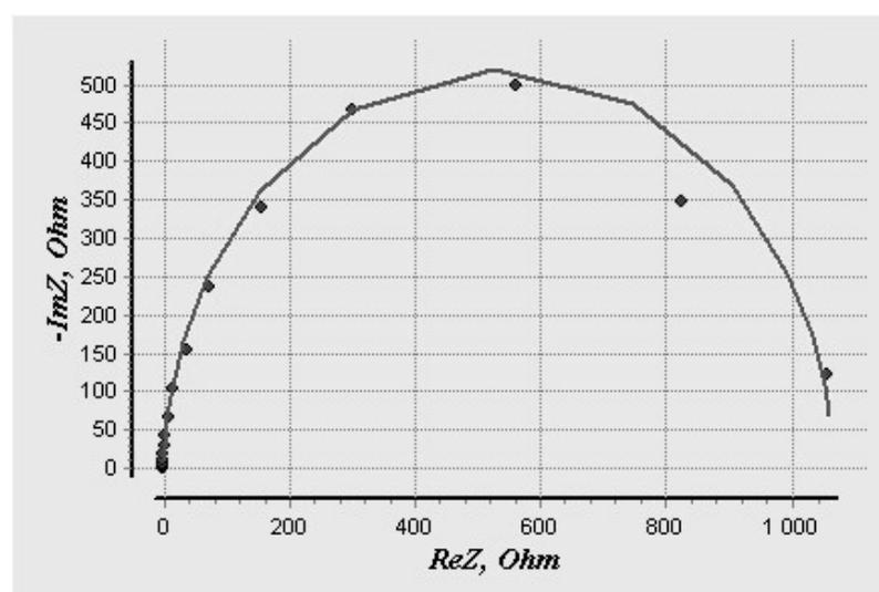
**Fig. 3.** An example of the Nyquist chart for a sample of the base material 7020M
