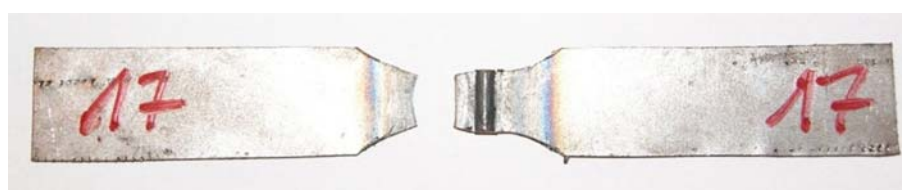
Fig. 11. Exemplary specimen after completing the tensile test
