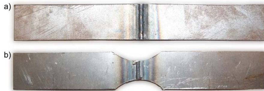
Fig. 7. Specimens prepared for tensile strength testing
