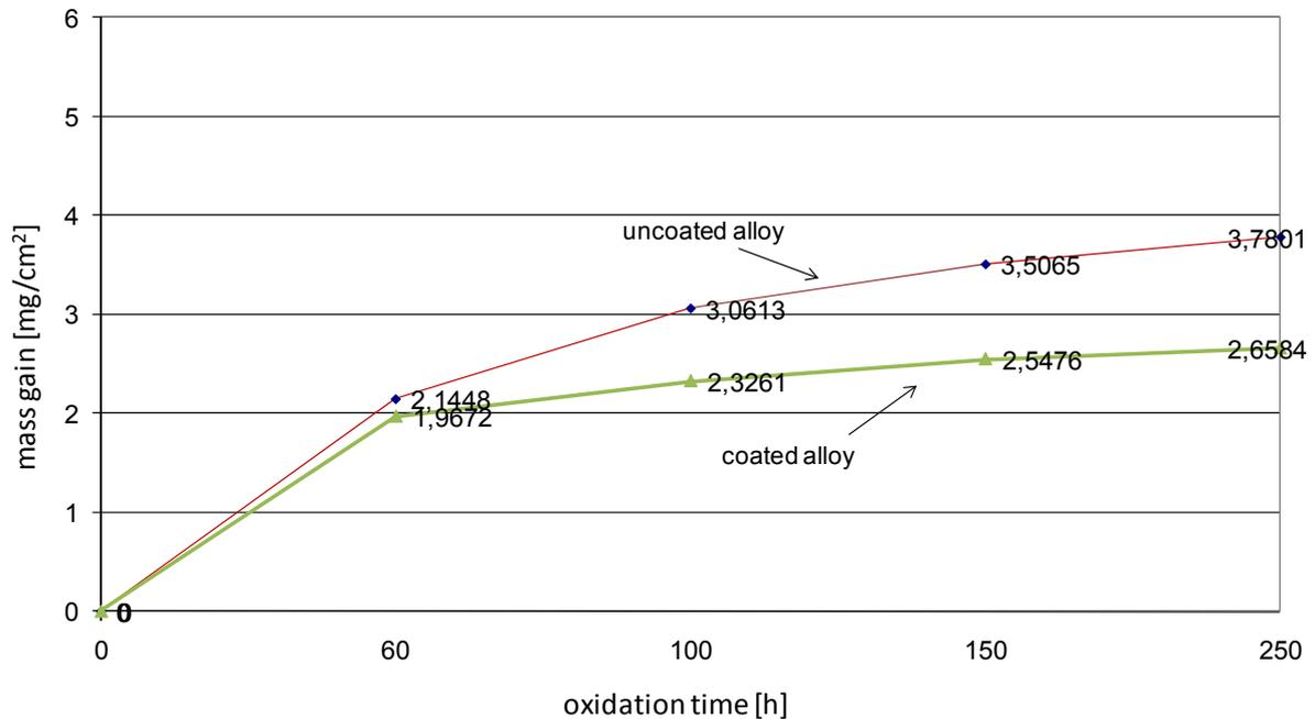
Fig. 2. The mass change of Ti-46Al-7Nb-0.7Cr-0.1Si-0.2Ni oxidized isothermally at 900°C
