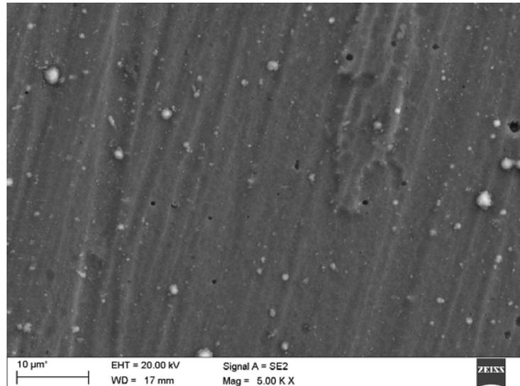
**Fig. 1.** SEM microphotograph for the surface of an as-deposited SiO<sub>2</sub> coating on a  $\gamma$ -TiAl specimen
