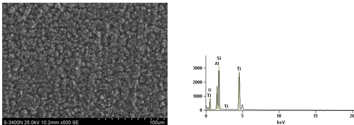
Fig. 3. SEM microphotograph for the surface of a SiO<sub>2</sub>-coated TiAl specimen after isothermal oxidation at 900°C in air and EDX analysis results of the surface
