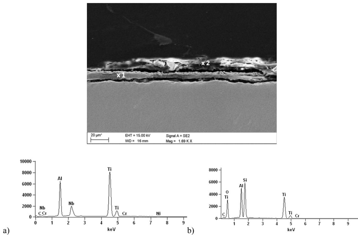
**Fig. 5.** Cross-section of the SiO<sub>2</sub> coated specimen of TiAl alloy after isothermal oxidation and EDX analysis results (a) in point #1, (b) in point #2
