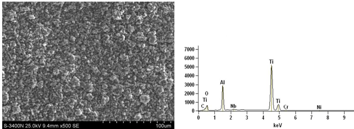
**Fig. 4.** SEM microphotograph for the surface of a uncoated TiAl specimen after isothermal oxidation at 900°C in air and EDX analysis results of the surface
