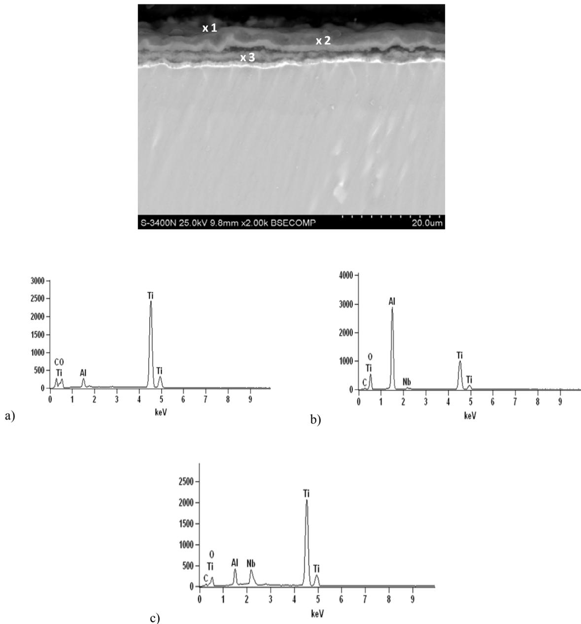
**Fig. 6.** Cross-section of the uncoated specimen of TiAl alloy after isothermal oxidation and EDX analysis results (a) in point #1, (b) in point #2, (c) in point #3
