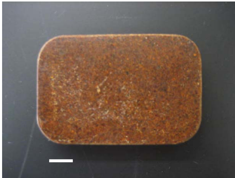
Fig. 2. Typical DDGS/phenolic compression-molded test specimen; scale bar indicates 10 mm (0.39 in)
