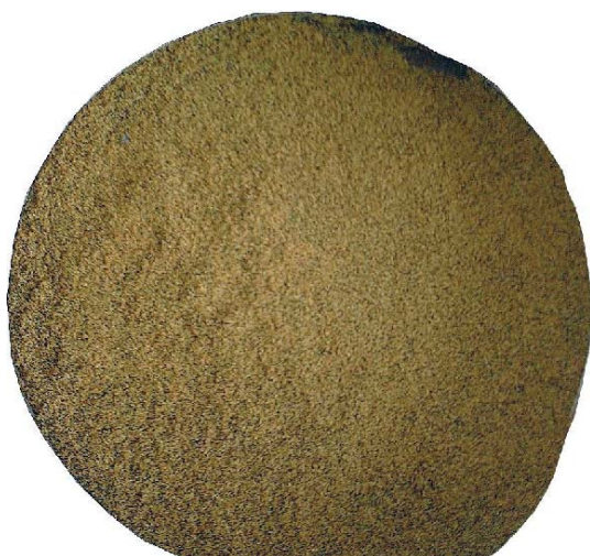
Fig. 4. Fraction 4 retained on the sieve with a mesh size 0.15 mm (left), fraction 5 retained on a sieve with mesh size 0.05 mm (right).
