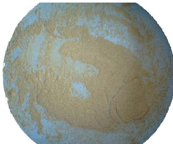
Fig. 4. Fraction 4 retained on the sieve with a mesh size 0.15 mm (left), fraction 5 retained on a sieve with mesh size 0.05 mm (right).
