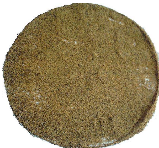
Fig. 3. Fraction 2 retained on the sieve with a mesh size 0.63 mm (left), fraction 3 retained on a sieve with mesh size 0.315 mm (right).
