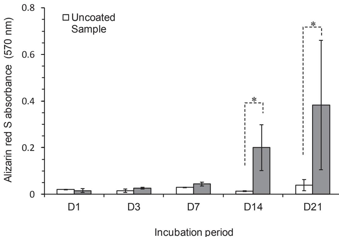
**Figure 2.** Comparison of cell mineralization on the surfaces of 20 uncoated and 20 coated (gray bars) titanium samples by Alizarin red S assay (error bars, standard deviation,  $n = 4$  per type per time point). Absorbance by the Alizarin red S at 570 nm, and D indicates the time of incubation in days. \* $P < 0.05$
