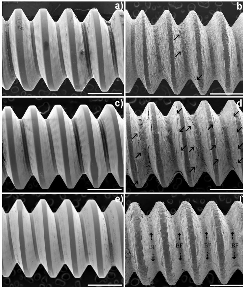
**Figure 5.** Scanning electron microscopy (SEM) image of uncoated and coated screws extracted from the bone. No detachment of the coating from the underlying screw is noted. Arrows indicate bone fragments (BFs). The amount and size of the BFs increased with increasing implantation periods. a) uncoated 7 weeks; b) coated 7 weeks; c) uncoated 12 weeks; d) coated 12 weeks; e) uncoated 24 weeks; and f) coated 24 weeks (magnification  $\times 100$ ). Scale bars represent 1 mm
