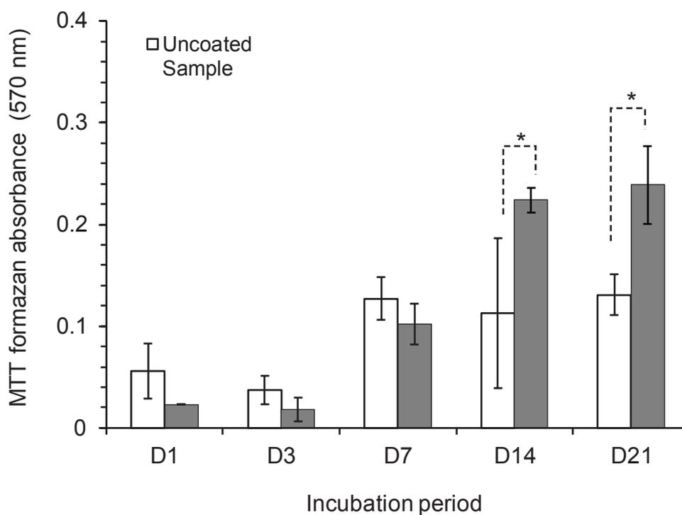
**Figure 1.** Comparison of cell proliferation on the surfaces between 20 uncoated and 20 coated (gray bars) titanium samples by methyl thiazolyl tetrazolium (MTT) assay (error bars, standard deviation,  $n = 4$  per type per time point). Absorbance by the MTT formazan chromophore at 570 nm, and D indicates the time of incubation in days. \* $P < 0.05$
